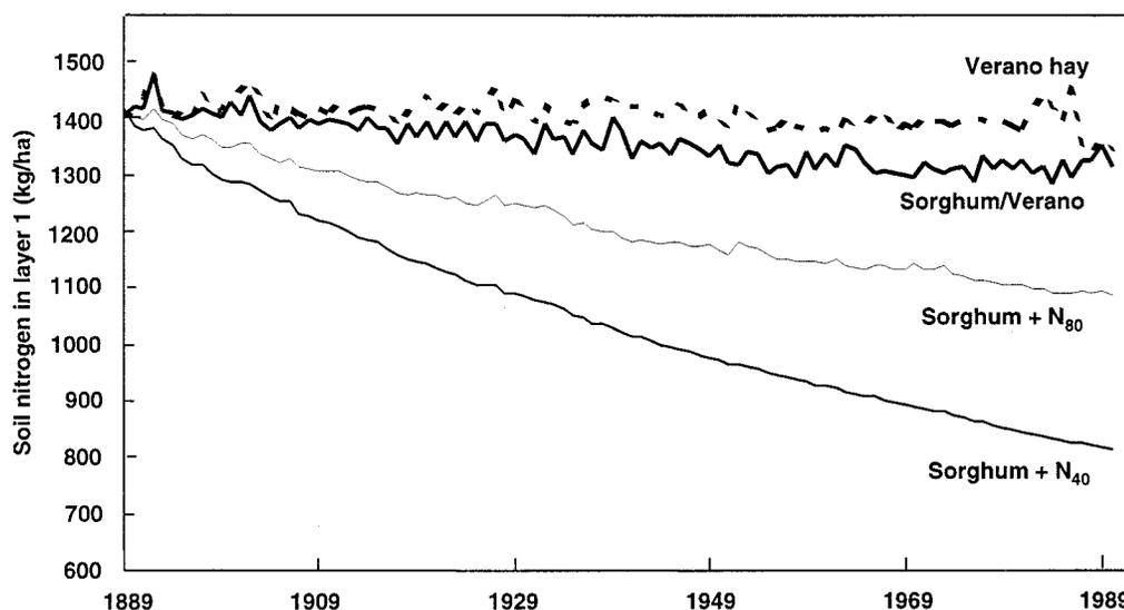
Figure 6. Simulated changes in the total soil nitrogen content of the top 0.15 m of soil over 1889–1990 for a number of alternative management options.
