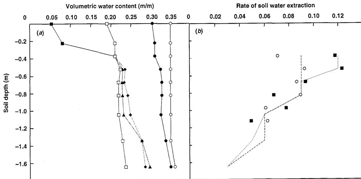
**Figure 1.** (a) Volumetric water content (VWC, m/m) describing soil saturation (○), drained upper limit (●), air dry (■), and the lower limits of water extraction for sorghum (□), maize (◆) and Verano (▲). (b) Rate of soil water extraction ( $kl$ ) measured for maize (■) and Verano (○) and the values used in APSIM modules for maize (—) and Verano (---). Error bars represent  $\pm$  s.e.
