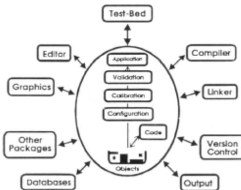
Figure 3. Programming environment for APSIM.
