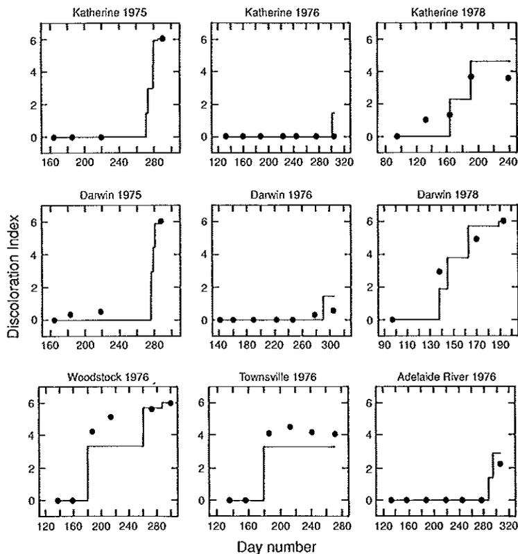
Fig. 2. Measured (●) and predicted (—) development of moulding.
